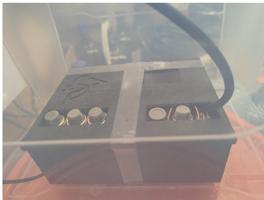
Figure 4: Data acquisition package and sensor array mounted inside closed system chamber for gas concentration monitoring during VOC reduction testing.
